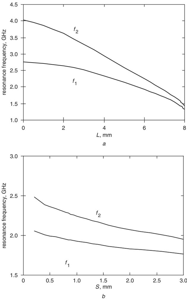
**Fig. 4** Mode resonance frequencies against slot length  $L$  and width  $S$  of the element of Fig. 2b for  $W=17$  mm on Duroid substrate with  $\epsilon_r=10.2$  and thickness 0.635 mm
