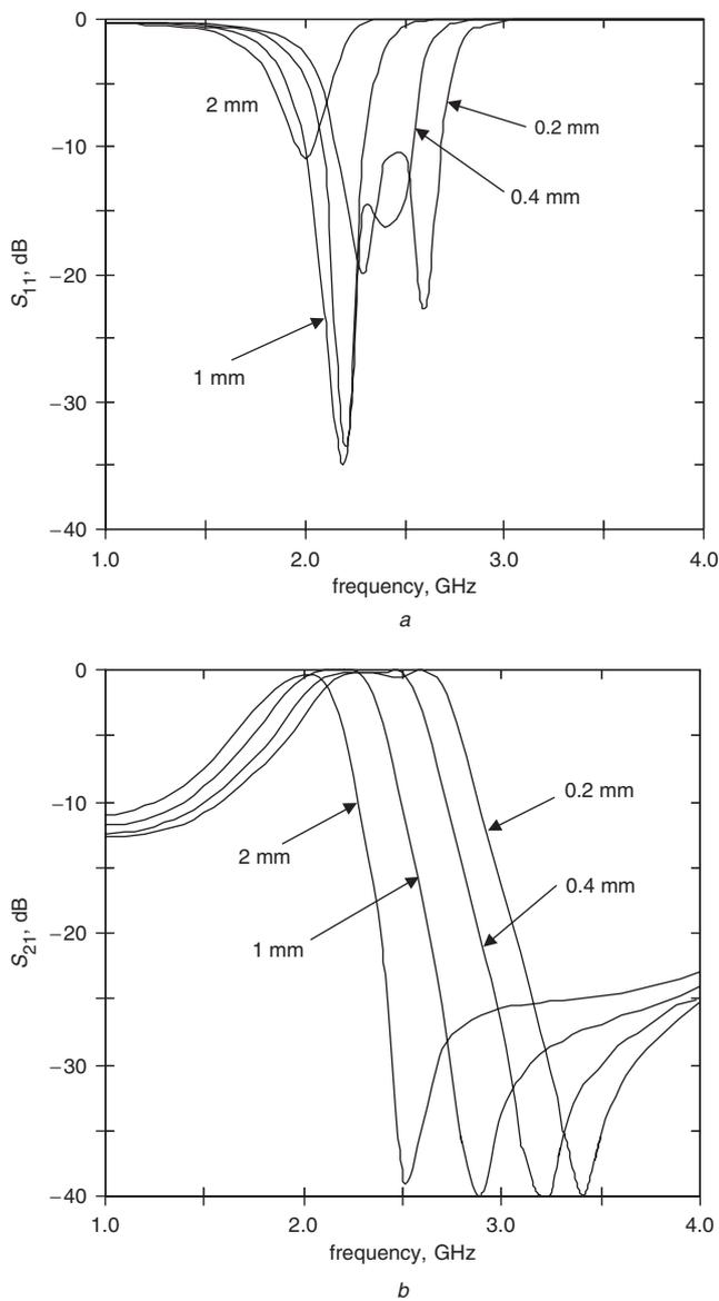
**Fig. 6** Simulated frequency response of dual-mode filtering behaviour for different values of slot width  $S$  with  $L=6\text{ mm}$ ,  $W=17\text{ mm}$ ,  $\epsilon_r=10.2$  and  $h=0.635\text{ mm}$
