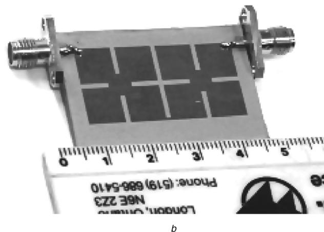
**Fig. 11** Photographs of the fabricated filters
