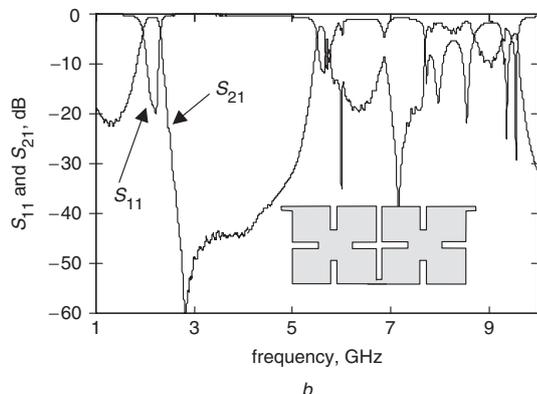
**Fig. 10** Simulations (based on IE3D) and experimental results of two cascaded elements four-pole filter
