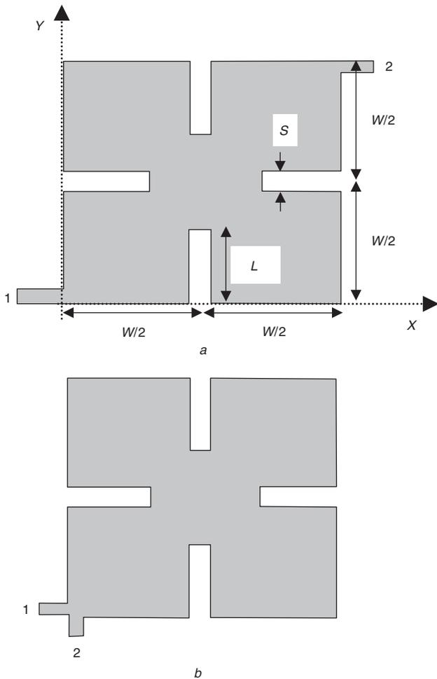
**Fig. 2** Dual-mode bandpass filter
