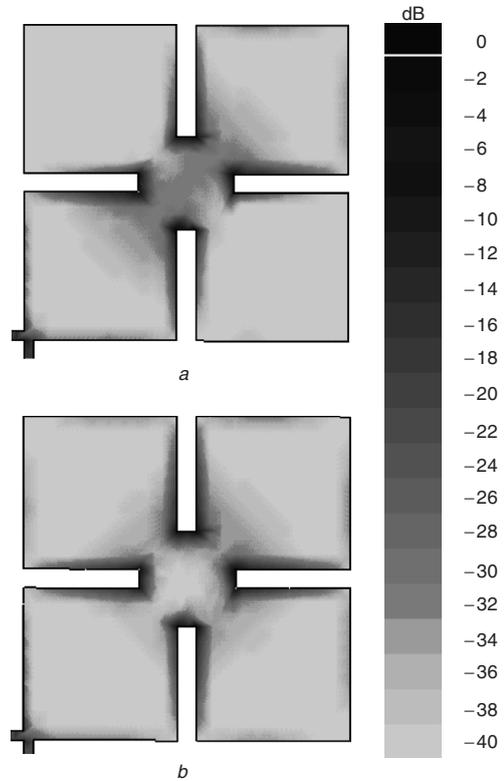
**Fig. 3** Simulated current density of the excited modes for  $W=17$  mm,  $L=6$  mm and  $S=1$  mm
