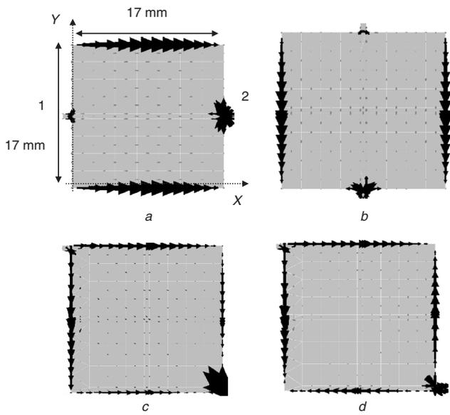
**Fig. 1** Current distribution of first three modes of square patch of side length of 17 mm on Duroid substrate with  $\epsilon_r=10.2$  and thickness 0.635 mm
