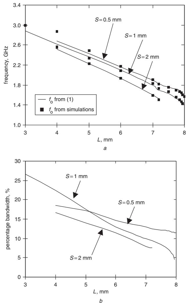
**Fig. 7** Variation of filter resonance frequency (a) and fractional bandwidth (b) against  $L$  for different values of  $S$
