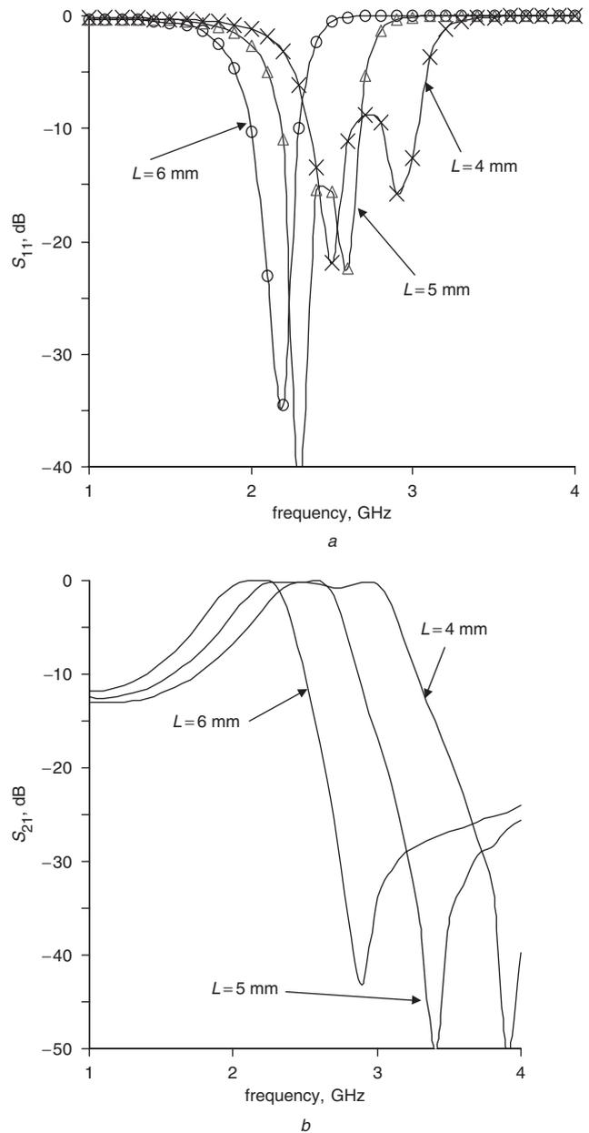
**Fig. 5** Simulated frequency response of dual-mode filtering behaviour for different values of slot length  $L$  with  $S=1$  mm,  $W=17$  mm,  $\epsilon_r=10.2$  and  $h=0.635$  mm
