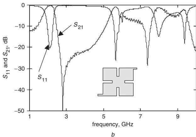
**Fig. 9** Simulations (based on IE3D) and experimental results of a one-element two-pole filter
