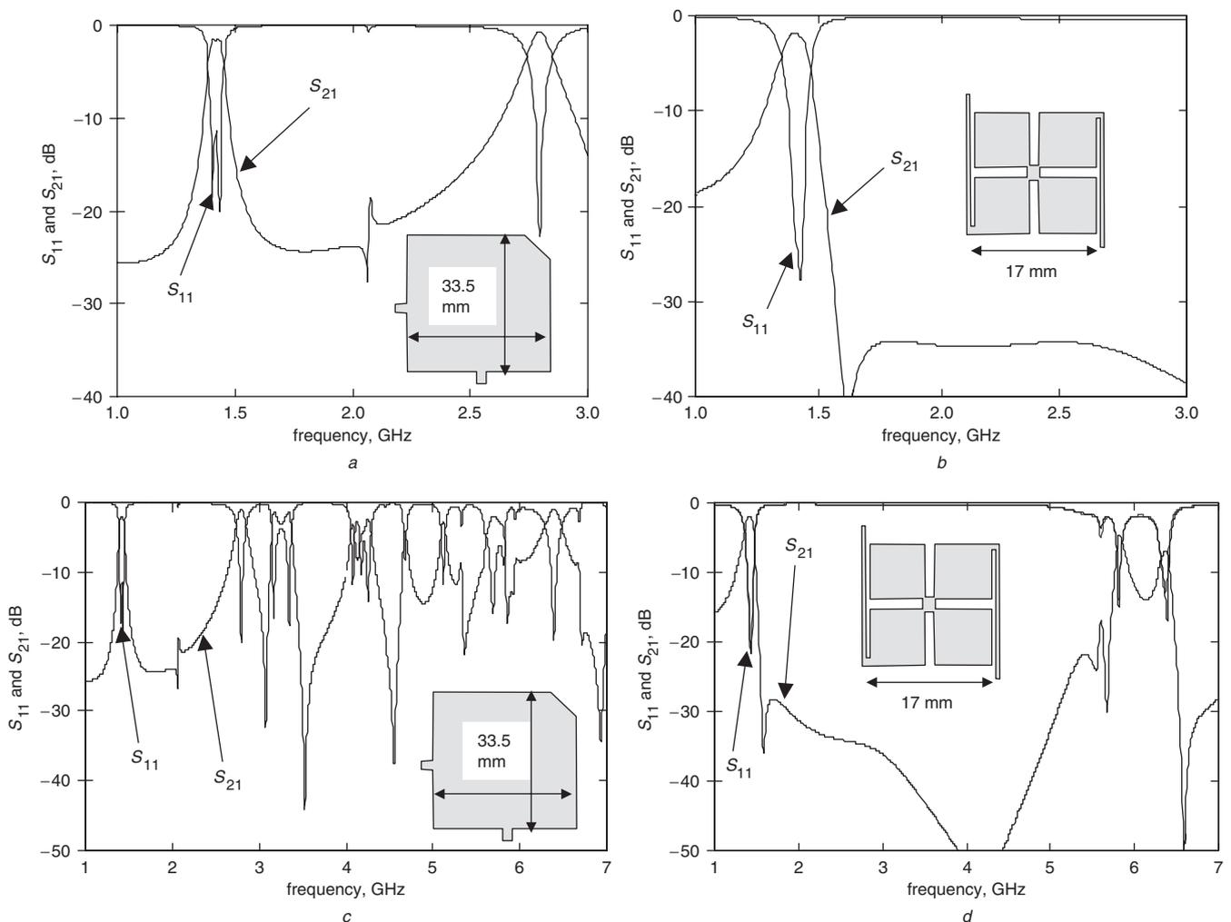
**Fig. 8** Simulation results of two filters: conventional degenerate dual-mode cut-corner  $33.5 \times 33.5$  mm square patch (a, c), and proposed nondegenerate dual-mode  $17 \times 17$  mm filter (b, d), designed at about 1.425 GHz on Duroid substrate with  $\epsilon_r = 10.2$  and thickness 0.635 mm
