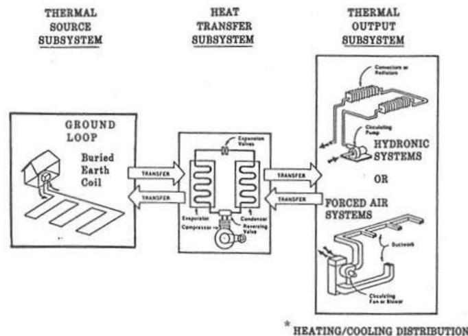
Figure 1: Basic Ground Source Heat Pump Components <sup>[5]</sup>
