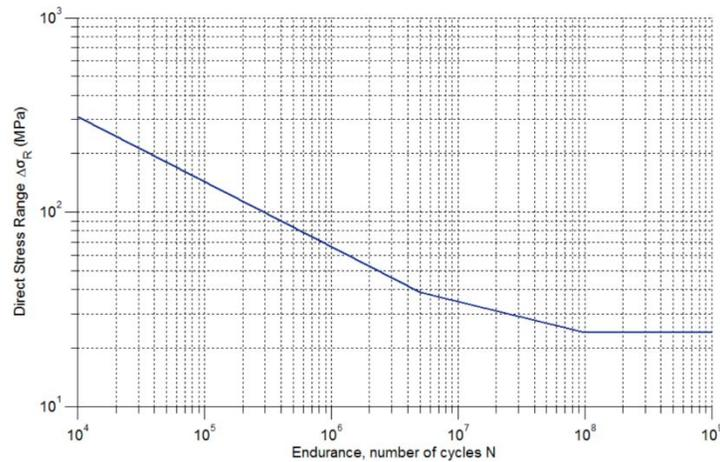
Figure 8. Direct Stress Range over number of cycles for detail type C
