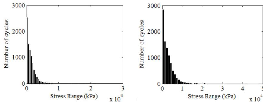
Figure 6. Annual Stress Range Spectra - Detail Type F – Tower [A] and Tower [B]
