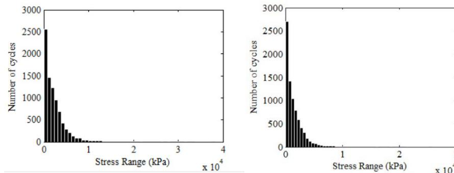
Figure 4. Annual Stress Range Spectra - Detail Type C – Tower [A] and Tower [B]
