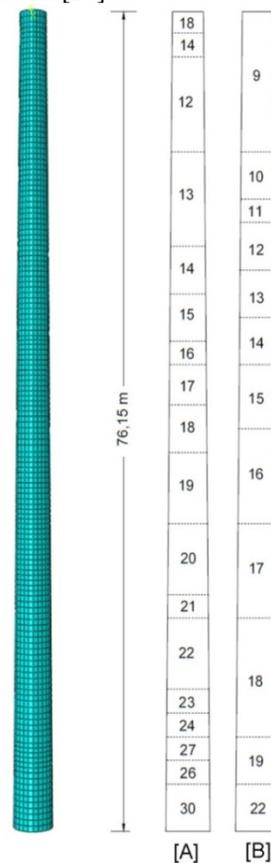
Figure 1. Shell thicknesses of investigated towers [A] and [B]
