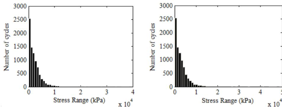
Figure 7. Annual Stress Range Spectra - Detail Type B – Tower [A] and Tower [B]
