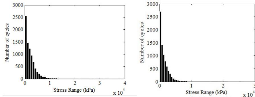
Figure 5. Annual Stress Range Spectra - Detail Type L – Tower [A] and Tower [B]
