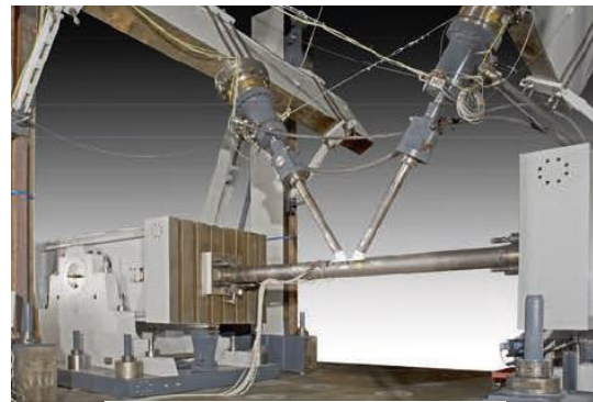
Figure 6. View of K-joint [32].
