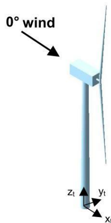
Figure 1: Tower-base coordinate system [3]
