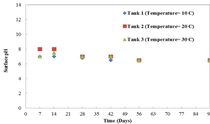
Figure 6 Effect of temperature on surface pH
