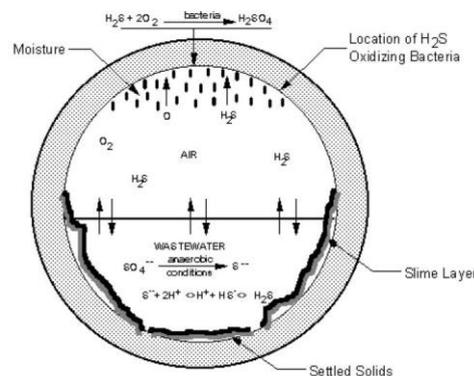
Figure 1 Sulphide generation in sewers [7]
