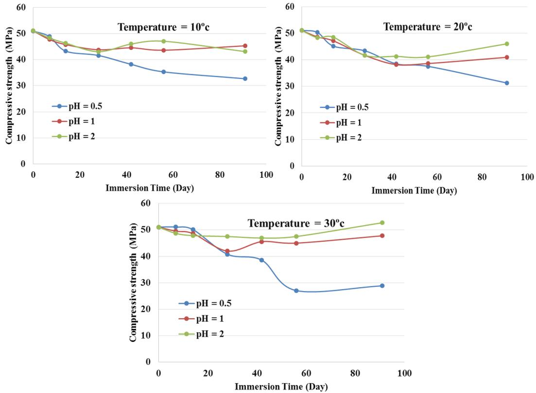
Figure 5 Compressive strength of the specimens in three different sulphuric acid solutions and three temperature
