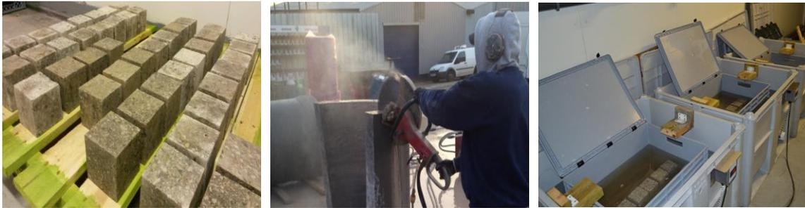
Figure 2 Sample preparation and acid bath stage
