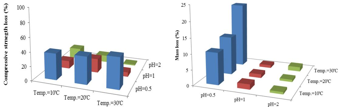
Figure 7 Variation in compressive strength loss and mass loss after 91 days experiment
