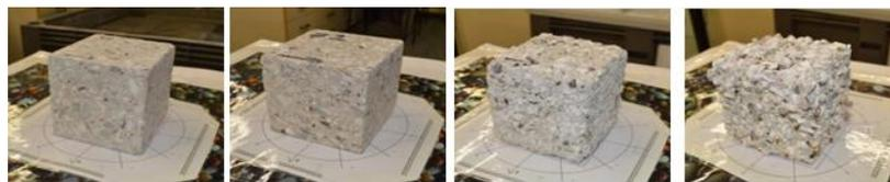
Figure 4 (a) original sample, (b) to (d) samples after 14, 56 and 91 days experiment, respectively.
