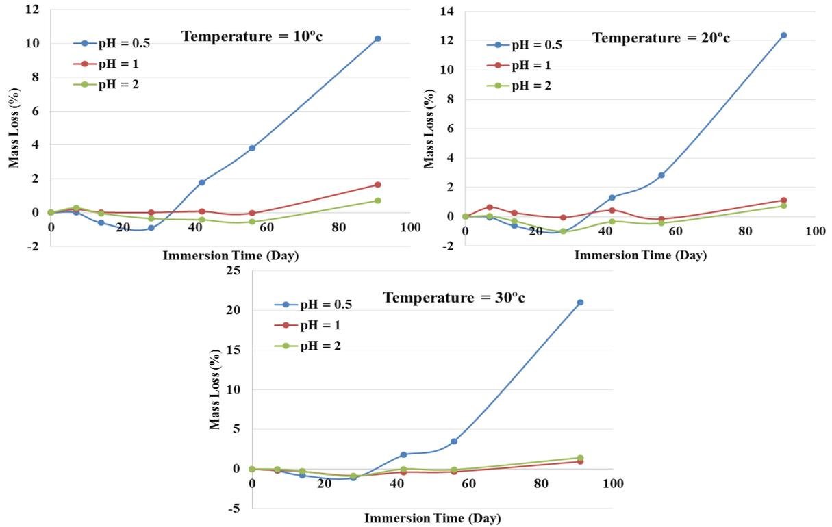
Figure 3 Mass loss of the specimens in three temperatures and three pH
