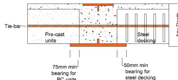
Figure 1: Schematic of USFBs with tie-bar shear connector [10]
