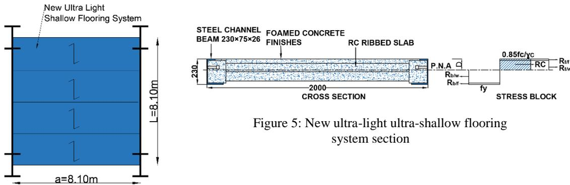
Figure 5: New ultra-light ultra-shallow flooring system section
