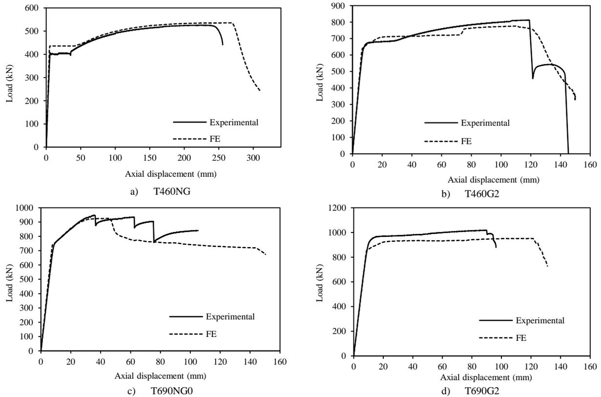
Figure 3. Tensile specimens - Comparison of numerical and experimental load-deformation response.
