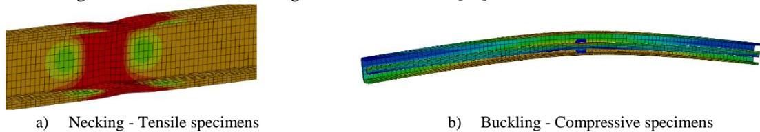
Figure 5. Failure modes.
