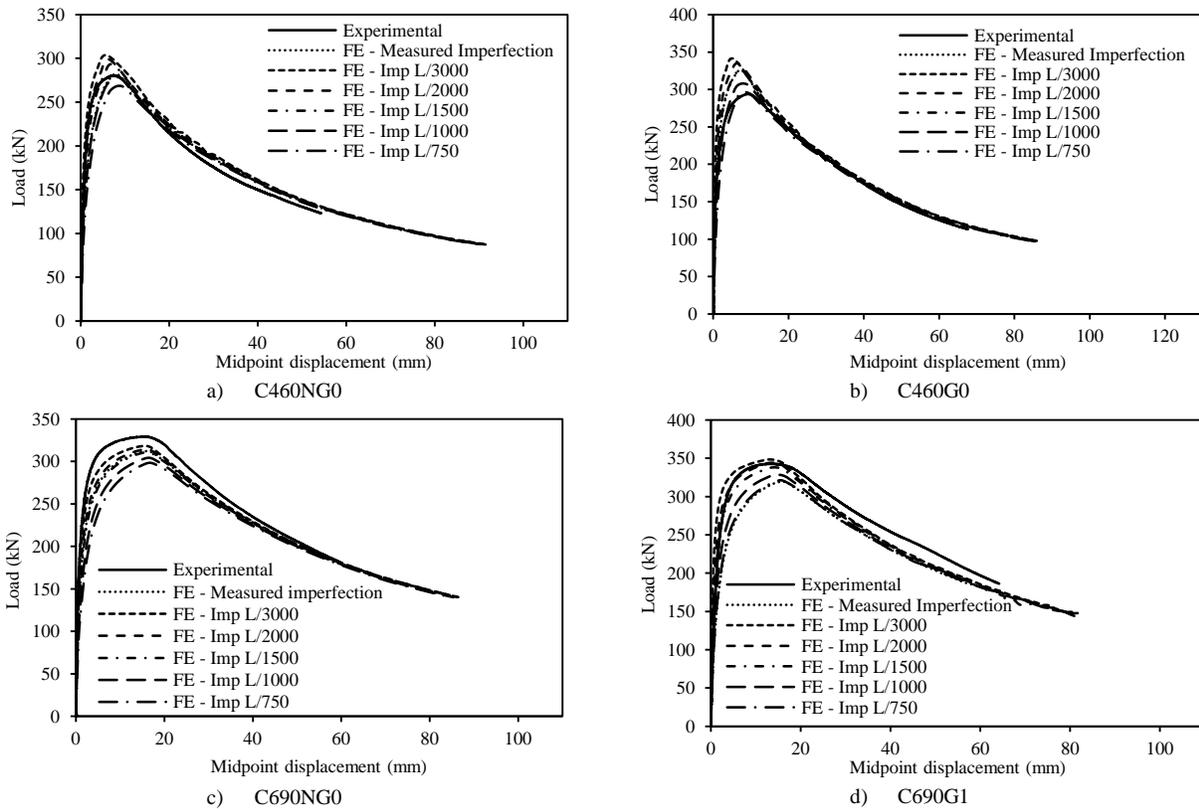
Figure 4. Compressive specimens - Comparison of numerical and experimental load-deformation response for six geometric imperfection magnitudes.
