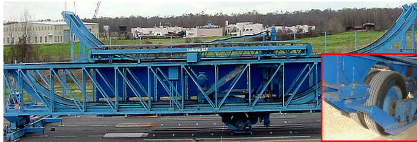
(b) Accelerated load facility
