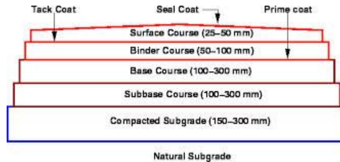
Figure 9. A cross section of a Pavement
