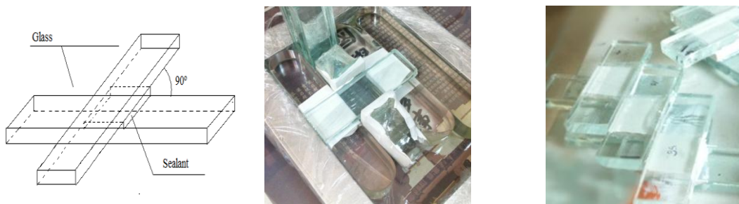
(a) Schematic diagram of test specimen (b) Moulding kits (c) Prepared cross-bonded specimens
