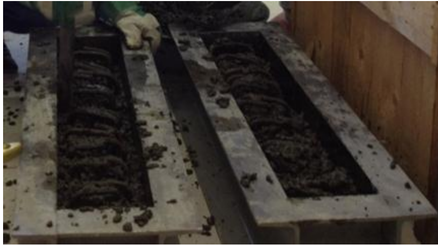
Figure 2. Casting of beams.
