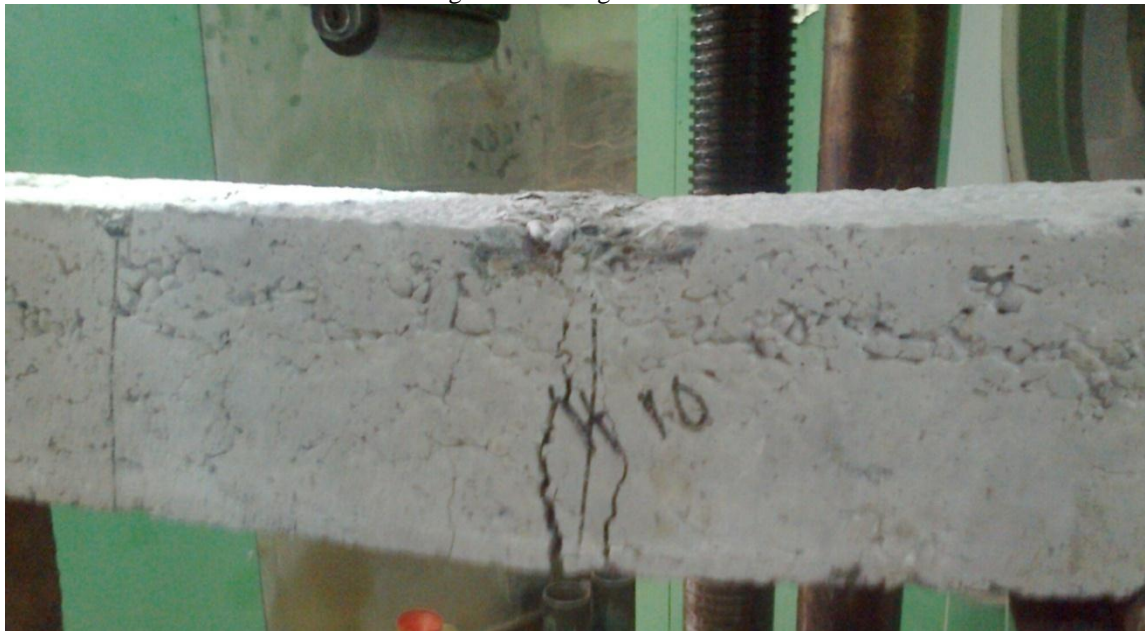
Figure 3. Flexural failure of H10 at 120 days.
