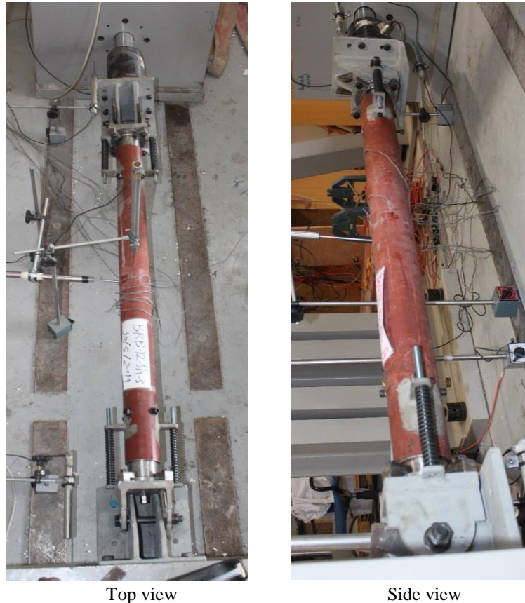
Figure 4. Instrumentation of BRB within the testing facility
