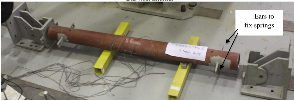
Figure 2. Actual photo of the hinge joint, end units, and restraining unit
