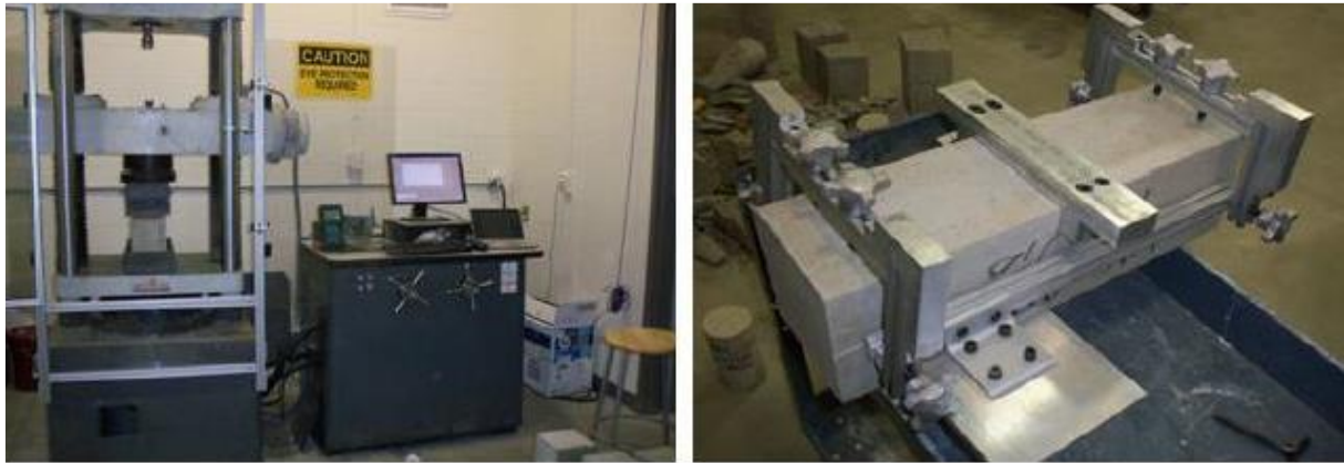
Fig. 1. Flexural performance test setup according to ASTM C1609
