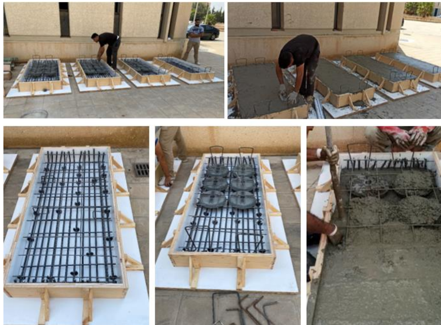
Figure 2. Portion of the preparation and casting practices of the specimens.
