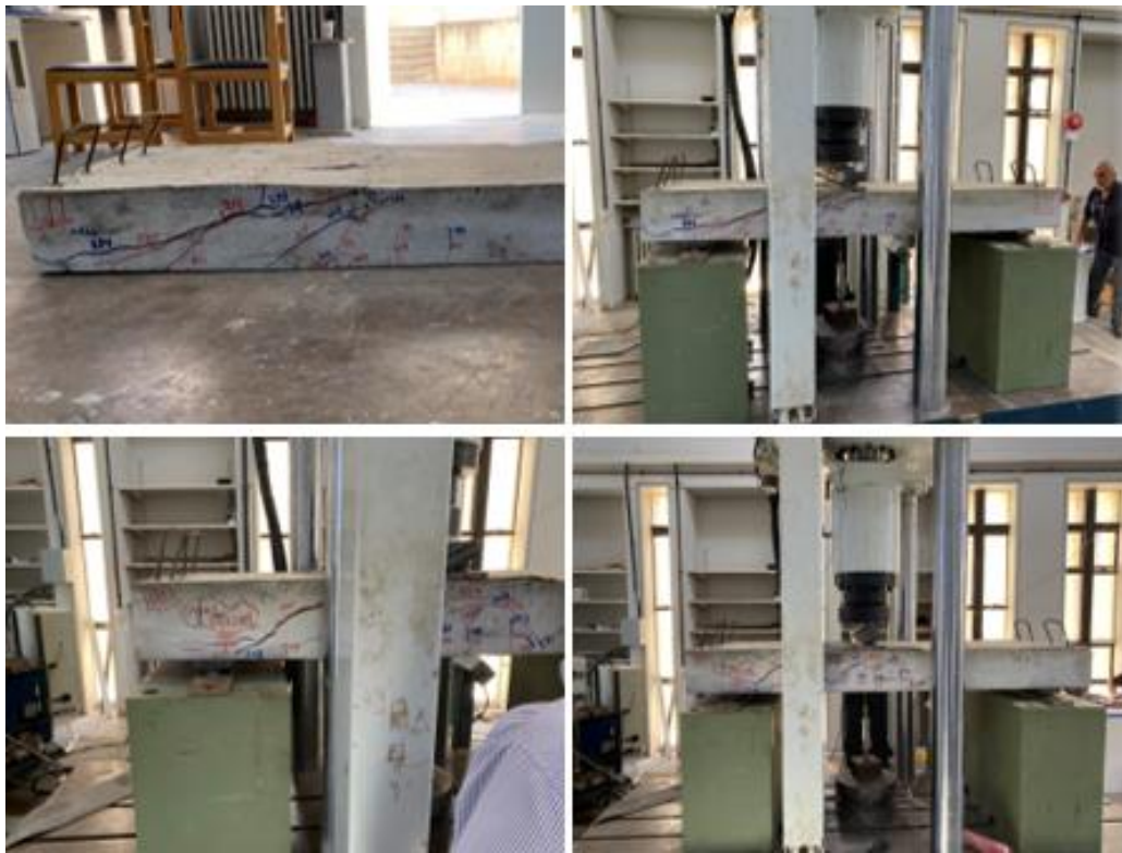
Figure 4. Typical shear failure and cracking patterns.
