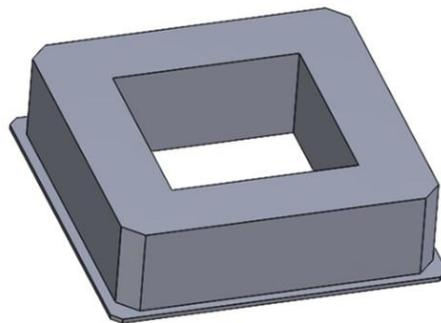
Figure 1. Platform of the barge-type floating wind turbine
