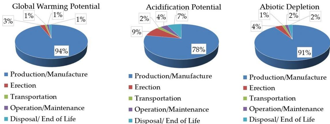
Figure 3. Contribution of each life cycle stage of the floating wind turbine to GWP, AP and ADPF
