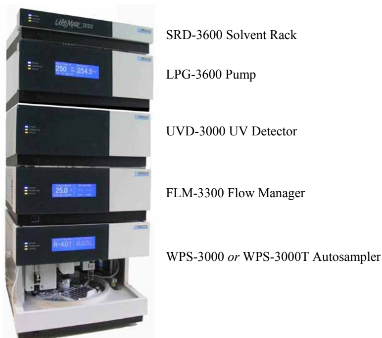
Fig. 10: Module arrangement for preconcentration
