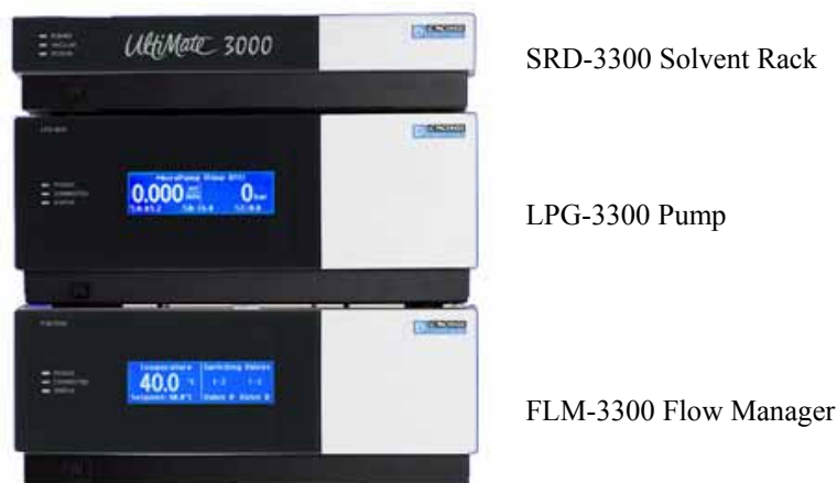
Fig. 4: Module arrangement for manual injection
